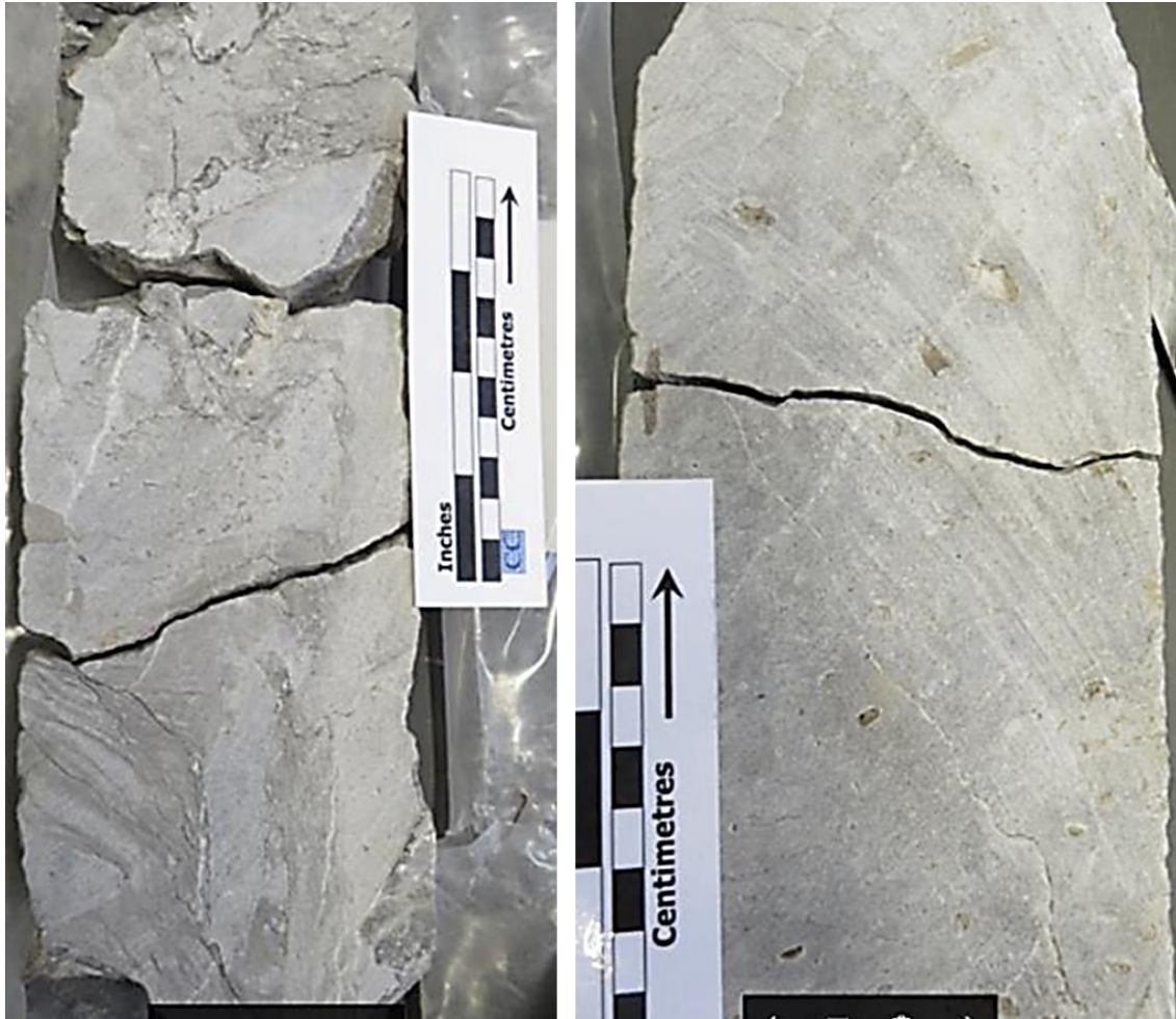
Figure 12-5: Left) Matrix-supported breccia with clasts of reefal carbonate in argillaceous matrix (1891.2 m). Right) Matrix-supported breccia with clasts of friable brown and green mudstone (1891.6 m).
